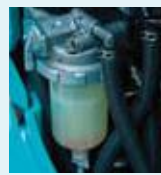
Pre fuel filter with built-in water separator
