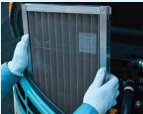
•30-mesh means that there are 30 holes formed by horizontal and vertical wires in every square inch of filter.
